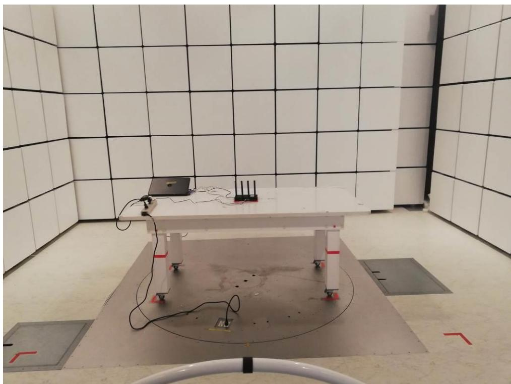
**Radiated Emissions Test Photos****30 MHz to 1000 MHz**
