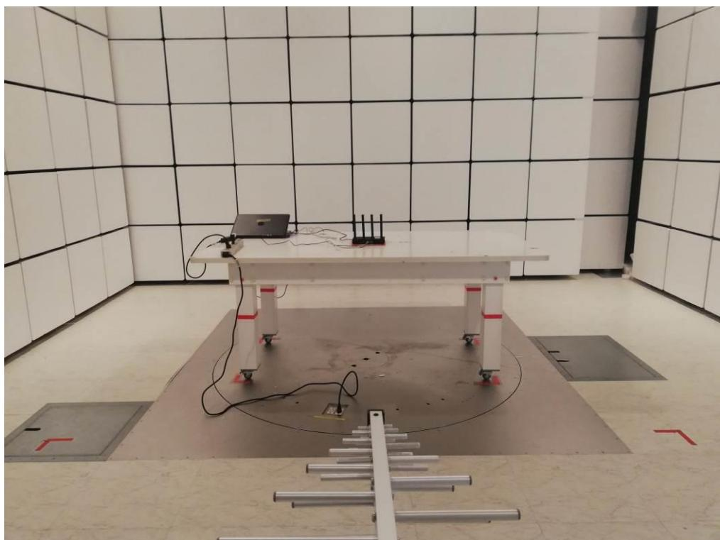
**Radiated Emissions Test Photos****Above 1000 MHz**
