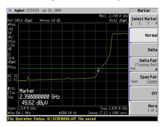
Detector mode: Peak Polarity: Horizontal
