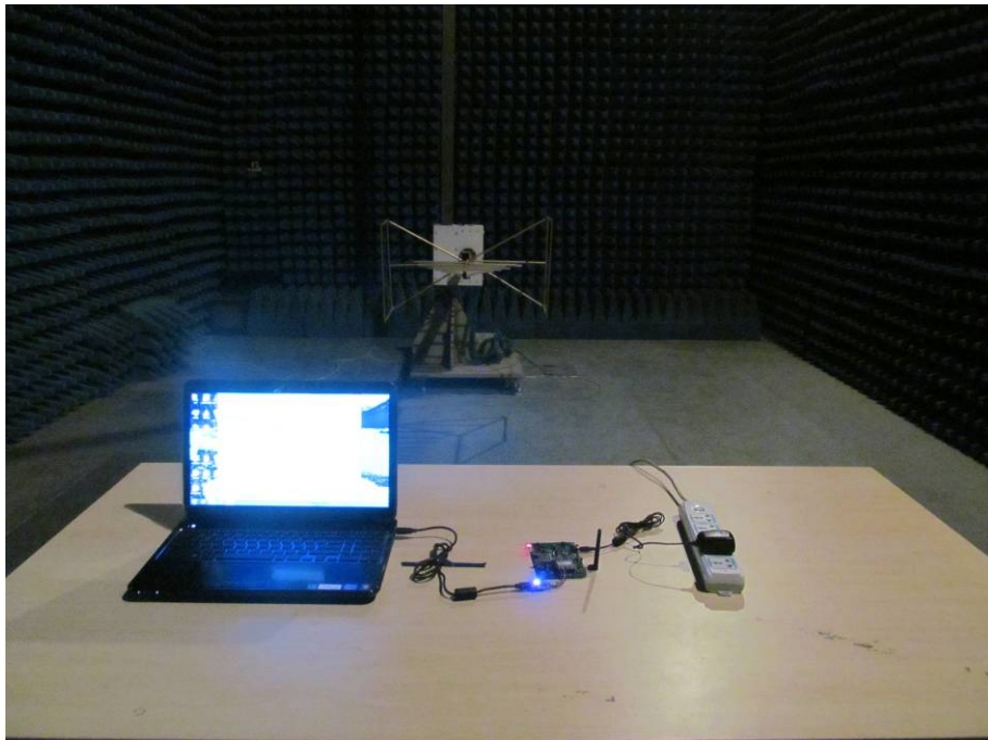
FCC RADIATED EMISSION TEST SETUP
