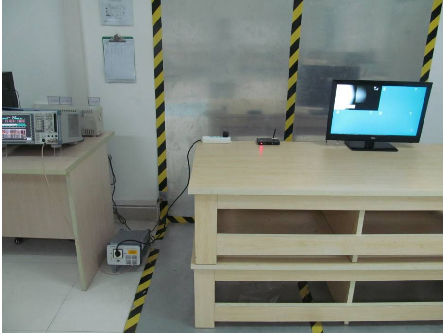
FCC RADIATED EMISSION TEST SETUP
