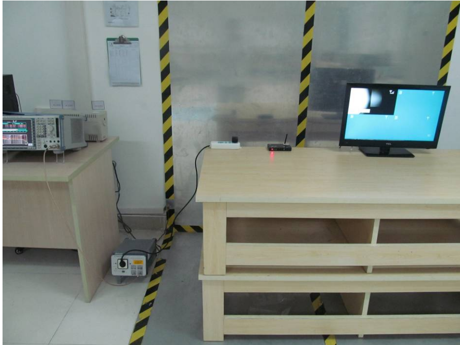
FCC RADIATED EMISSION TEST SETUP
