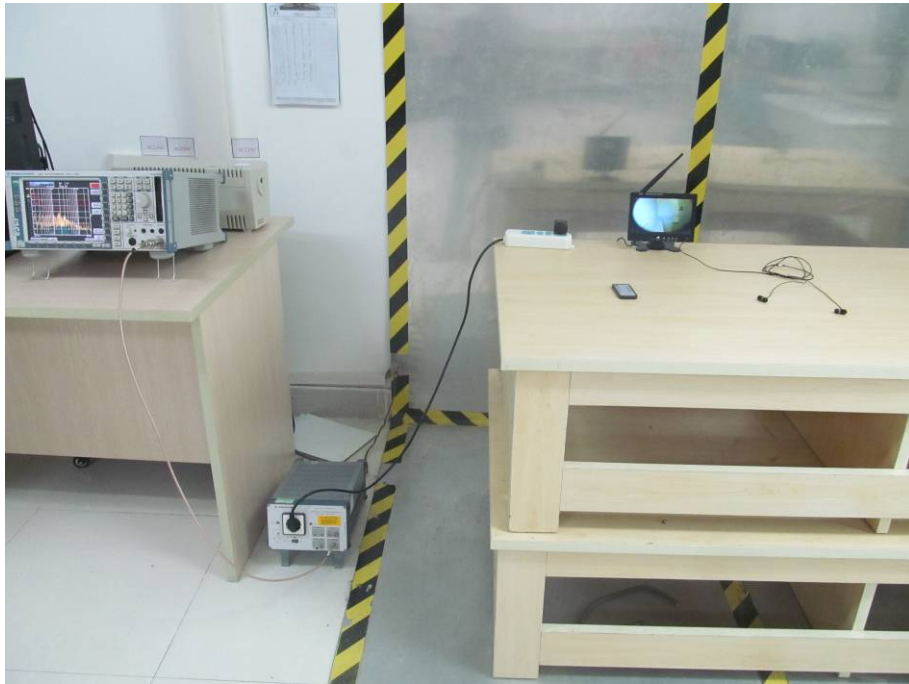
FCC LINE CONDUCTED EMISSION TEST SETUP
