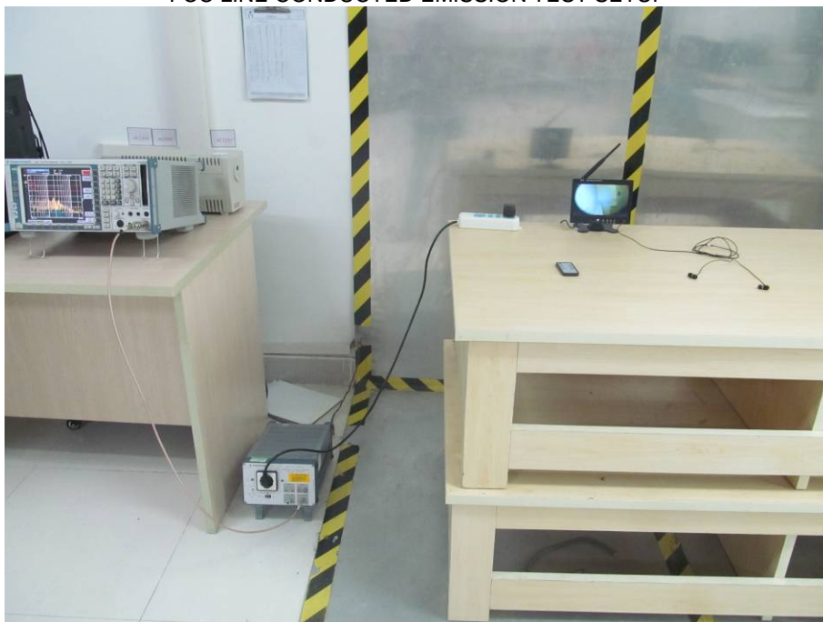
FCC RADIATED EMISSION TEST SETUP
