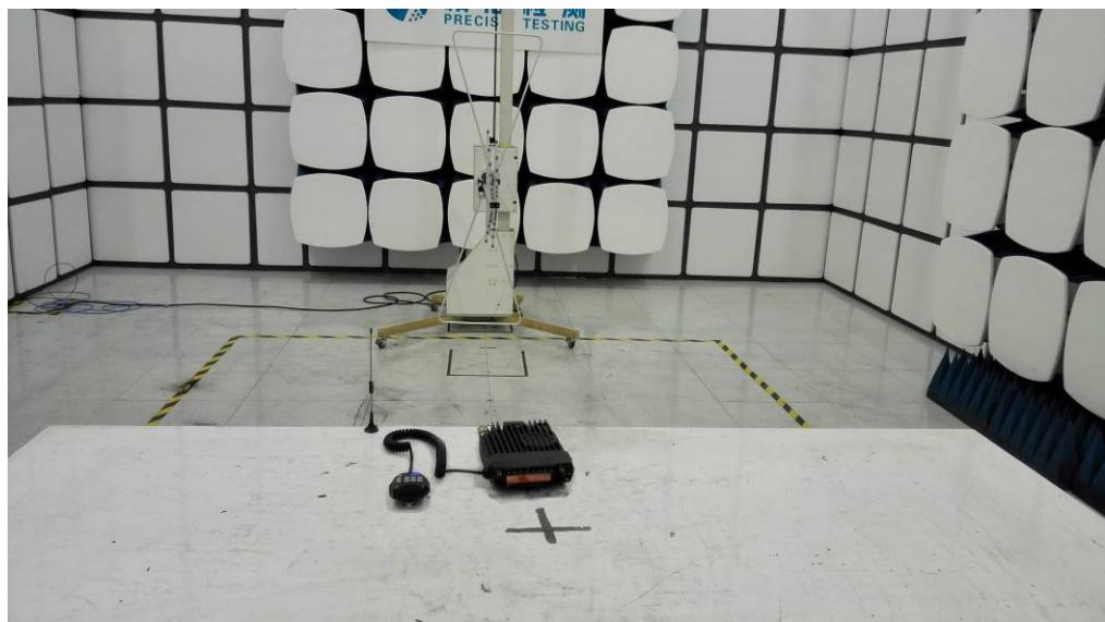
RADIATED EMISSION TEST SETUP ABOVE 1GHz
