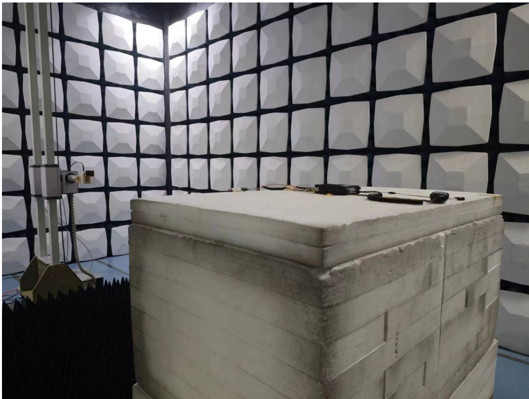
Radiated Emission 18-25GHz View
