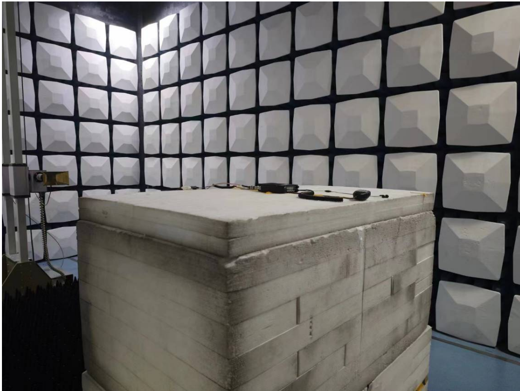
Radiated Emission 18-25GHz View
