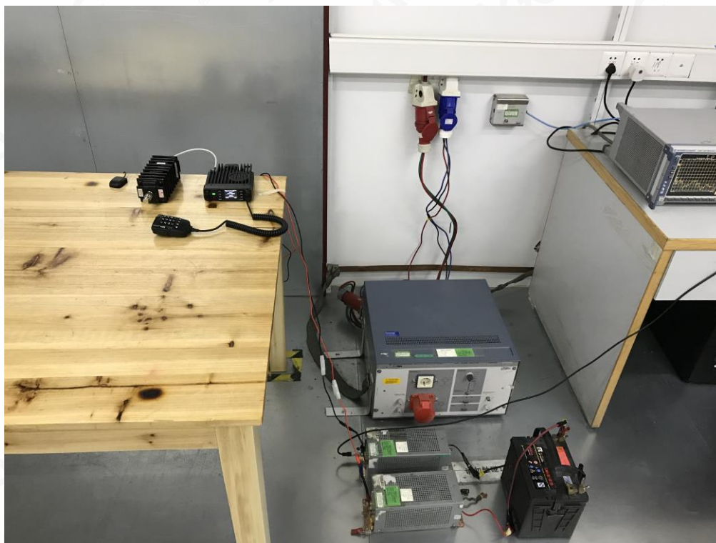
RADIATED EMISSION TEST SETUP-BELOW 1GHZ
