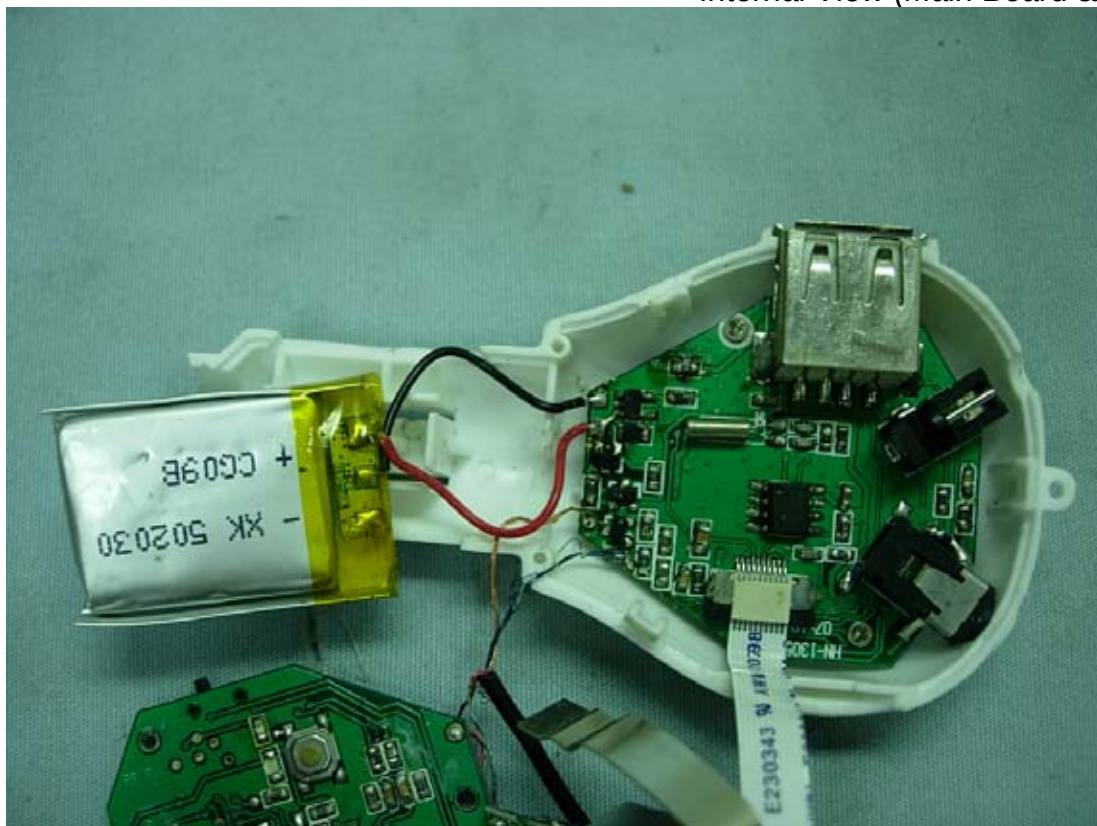
Figure 8 Internal View (Main Board & Battery)
