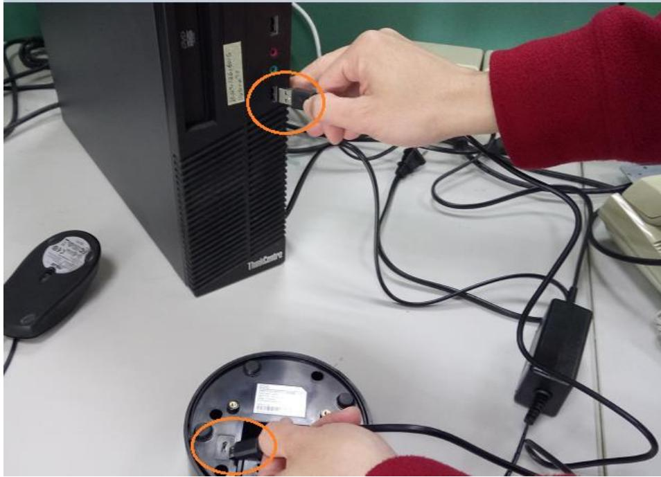
2. Press and hold the **Power** button. While holding the **Power** button, plug in the power cable.
