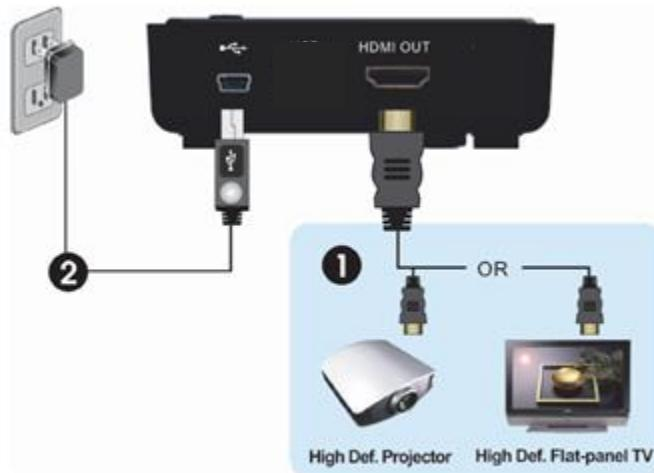
1. Connect the HDMI cable to the HDMI OUT jack of the receiver and to your HDTV set (or an HD projector).
