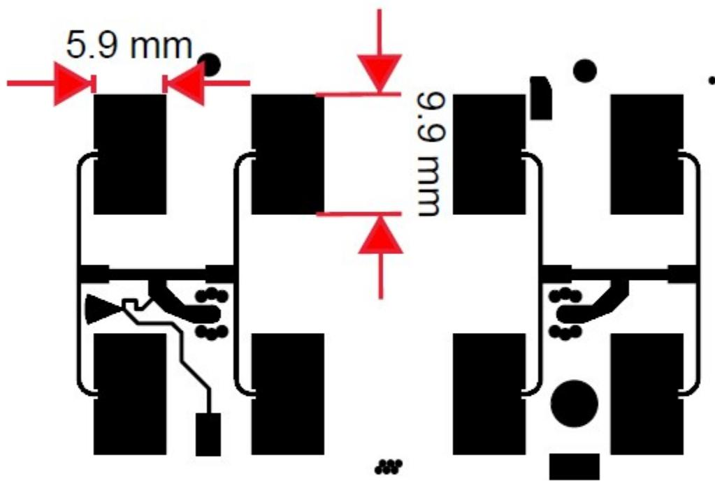
Each of the copper patches that comprise the transmit and receive antennas measures approximately 5.9mm by 9.9mm.
