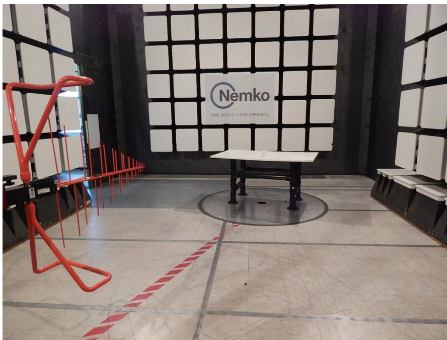
Figure 8.2-1: Radiated emissions setup photo – 30 to 1000 MHz
