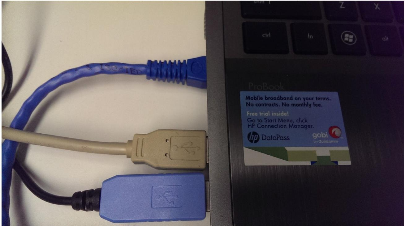
For reference, the Ember Adapter should have the USB cable and blue Ethernet cable connected as in the following picture
