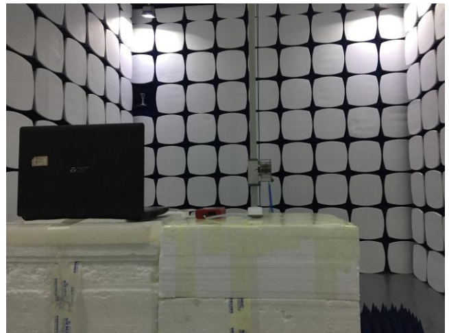
Radiated Spurious Emissions Test Setup Above 1GHz
