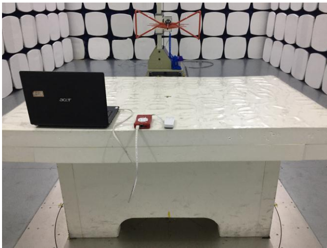
Radiated Spurious Emissions Test Setup Below 1GHz
