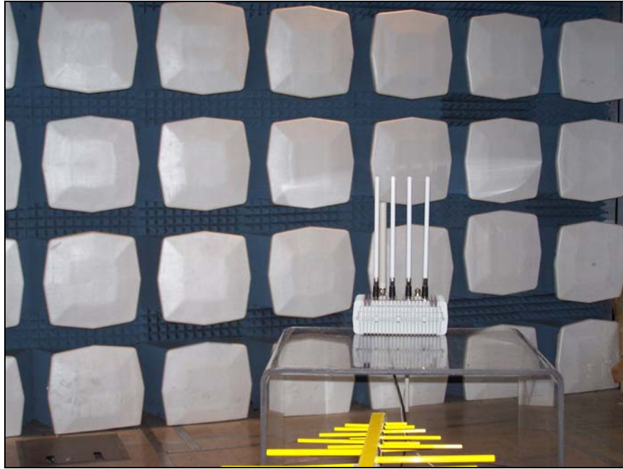
Photograph 2. Radiated Emission Test Setup, Below 1 GHz
