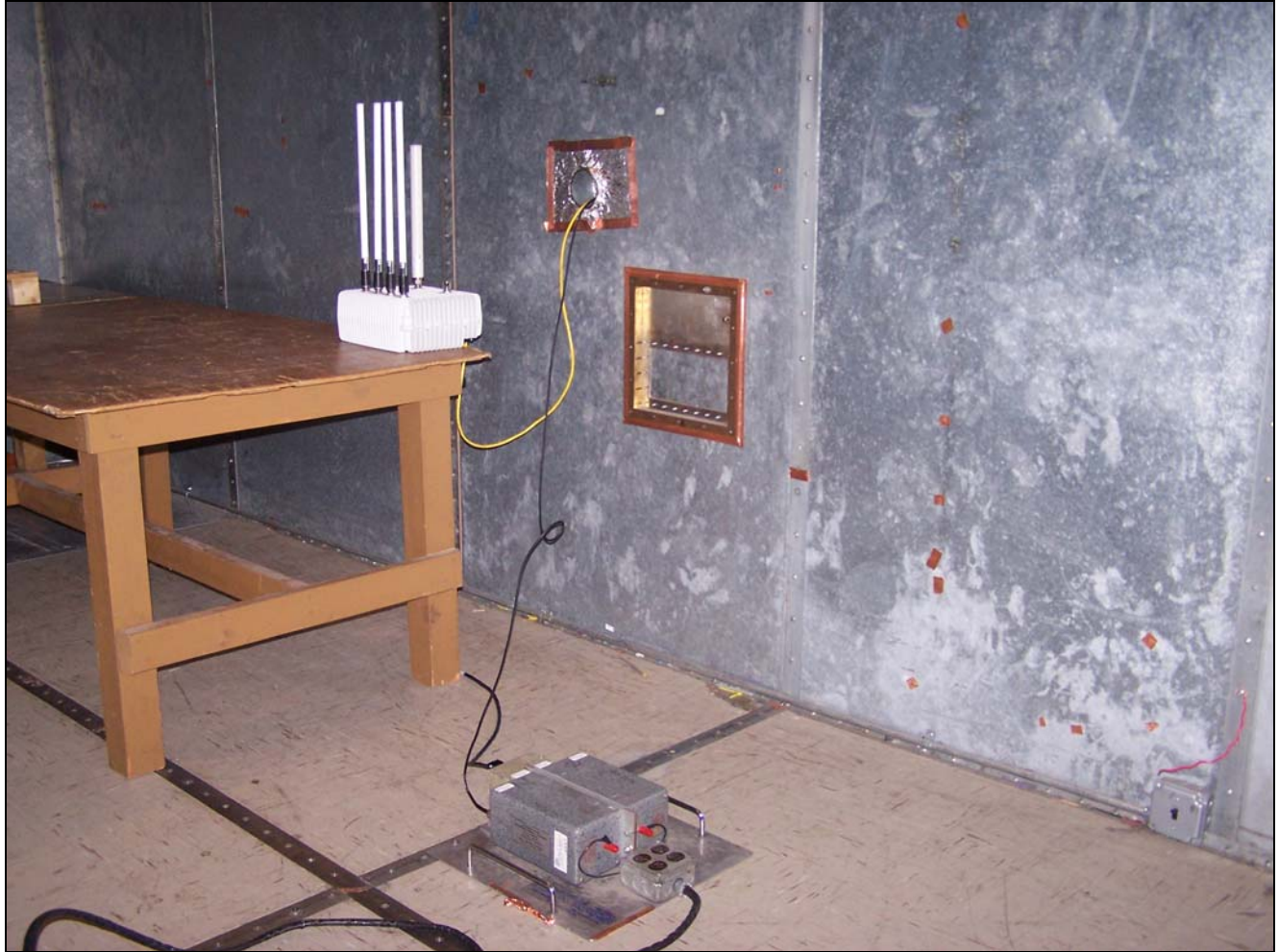
Photograph 4. Conducted Emissions Test Setup
