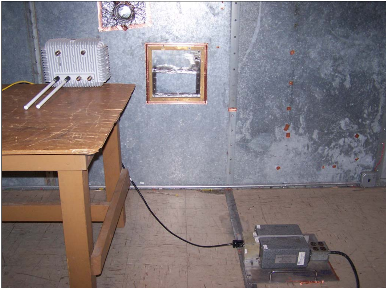
Photograph 1. Conducted Emissions Test Setup
