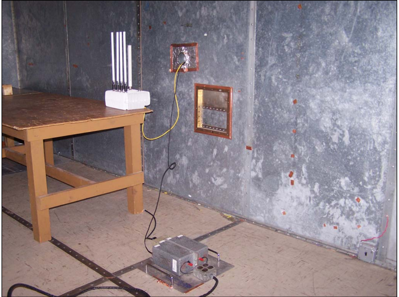
Photograph 4. Conducted Emissions Test Setup
