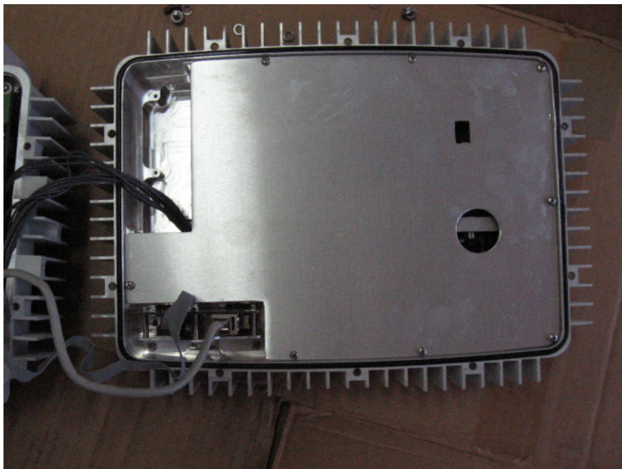
Figure 4 Bottom Cover With Heat Sink Plate Internal View
