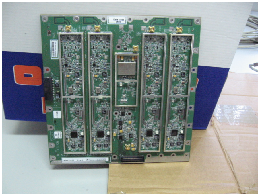
Figure 14 RF Card Component Side Without Shield
