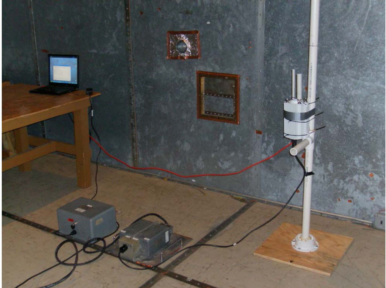
Photograph 1. Conducted Emissions Test Setup
