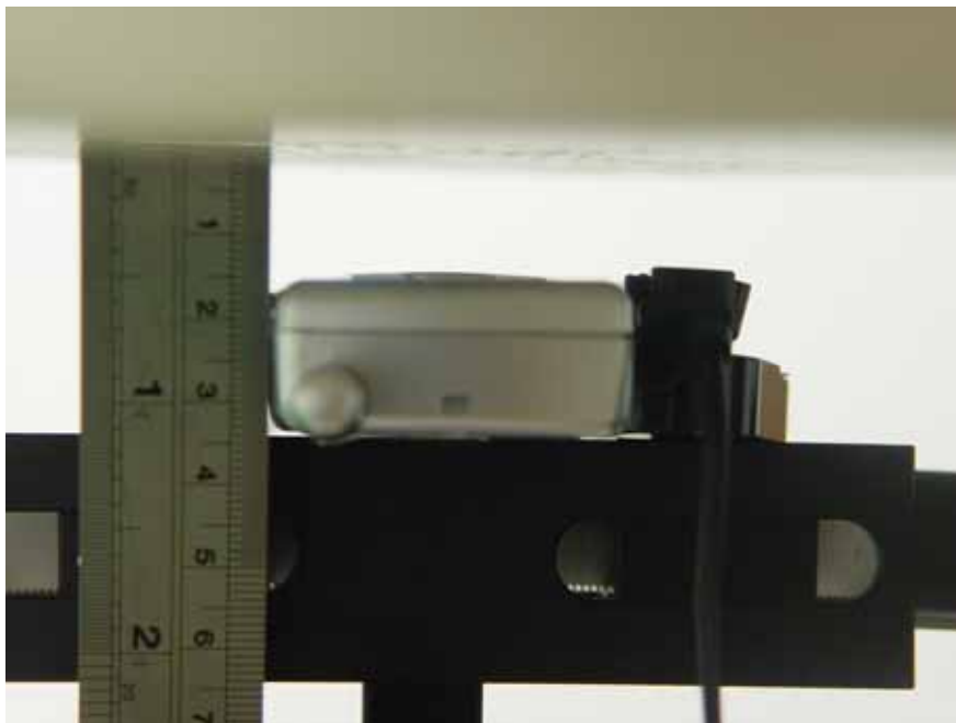
Fig. 9.7 Keypad Up with 1.5cm Gap
