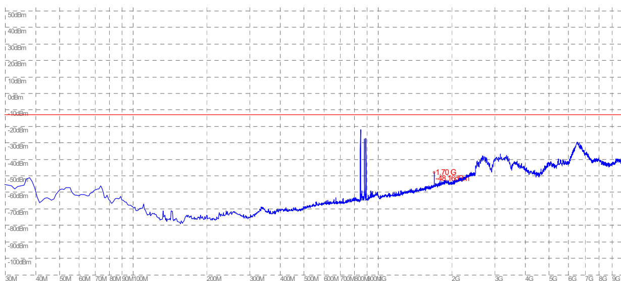
(Plot C.2: GSM 850MHz Channel = 251, Test Antenna Vertical)
