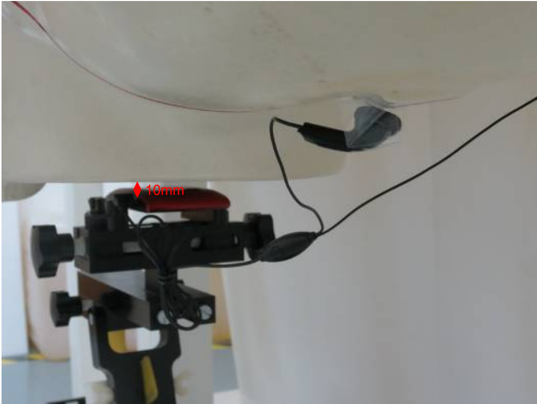
Picture 19: Back Side with Headset, the distance from handset to the bottom of the Phantom is 10mm
