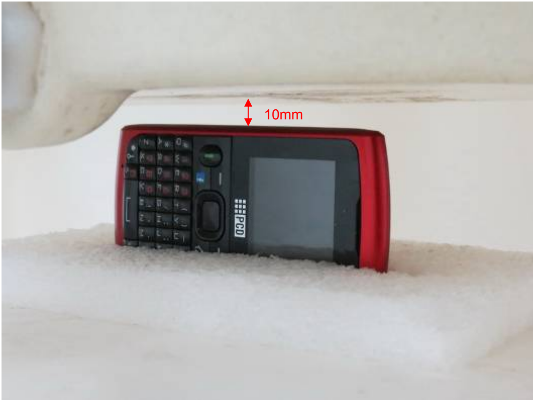
Picture 15: Left Edge, the distance from handset to the bottom of the Phantom is 10mm
