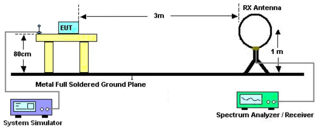
For radiated emissions from 30MHz to 1GHz
