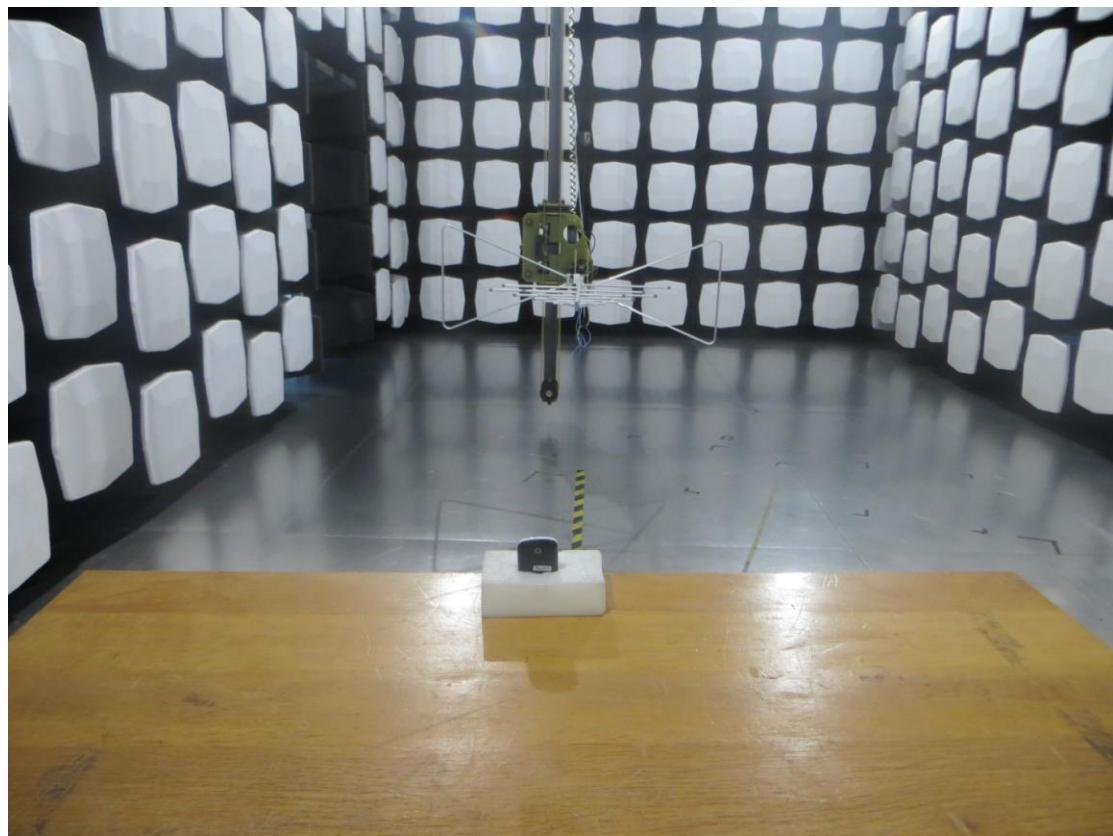
2. Part 15C Radiated emission above 1GHz
