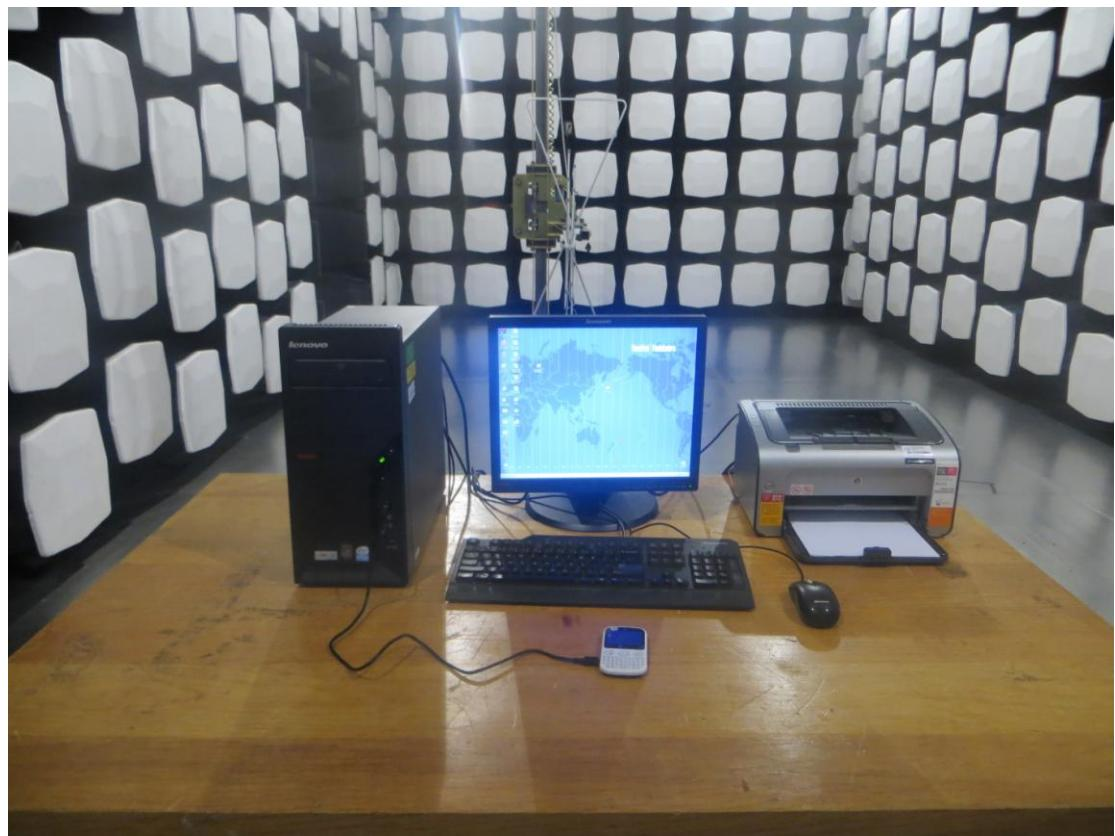
6. Part 15B Radiated emission (USB) above 1GHz
