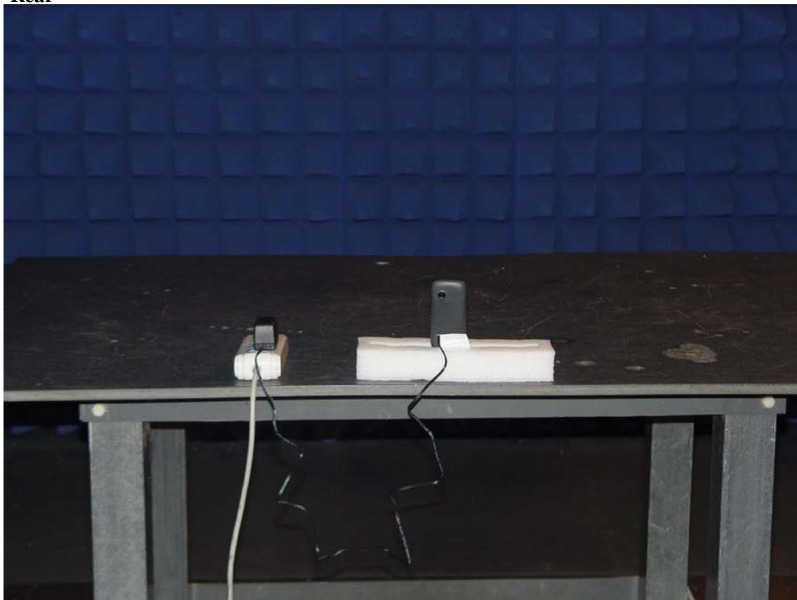
**FCC Part15C Radiated Emission below 1GHz****- Front**
