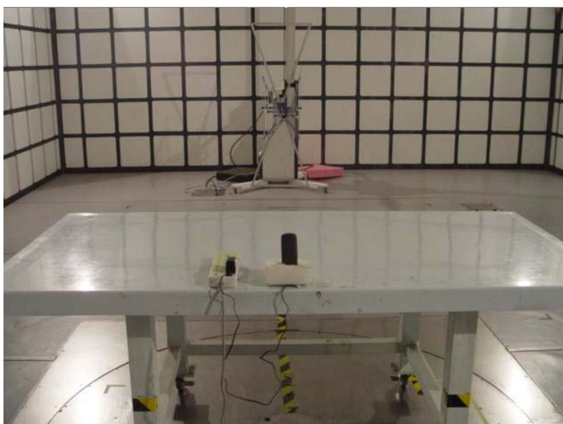
**FCC Part15C Radiated Emission above 1GHz****-Front**
