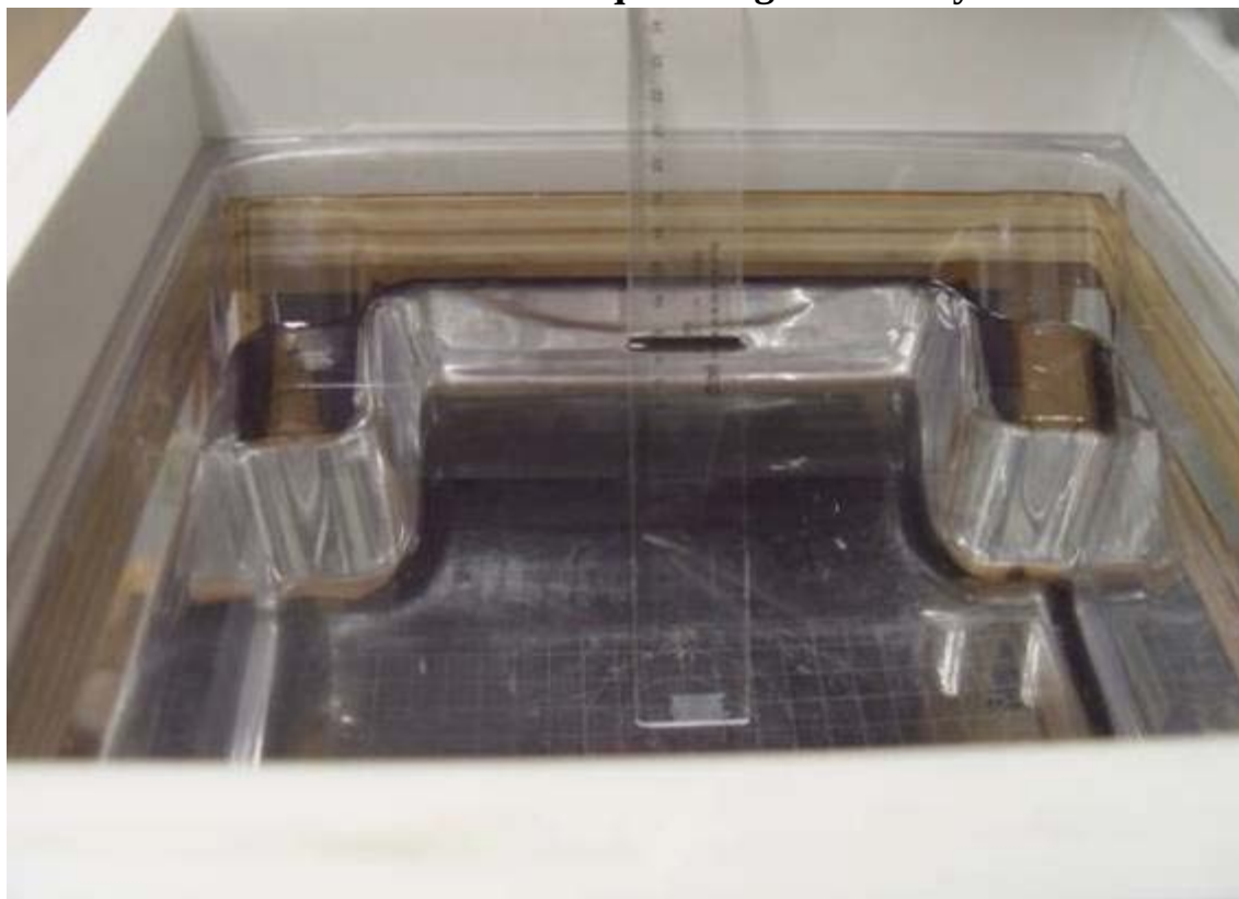
Photo of Liquid Height for Body SAR
