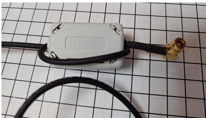
Wurth Ferrite N°742 711 12 with double cable routing inside.
