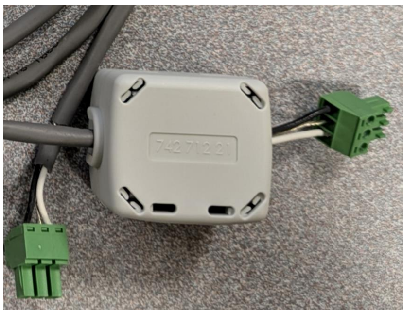
Wurth Ferrite N°742 712 21 with double cable routing inside
