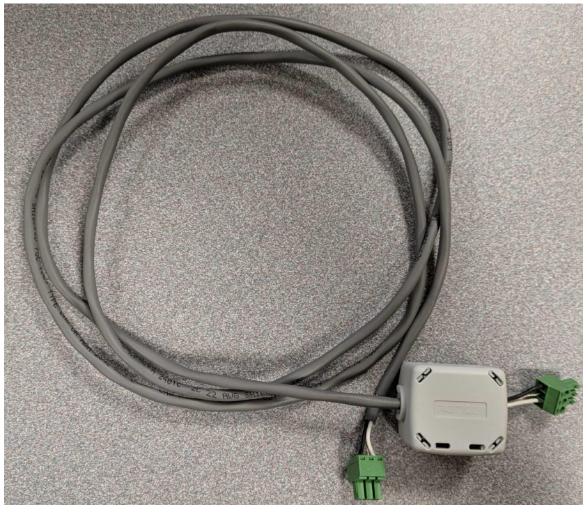
Cable for the ELM_1000035203 antenna liaison with Wurth Ferrites N°742 712 21
