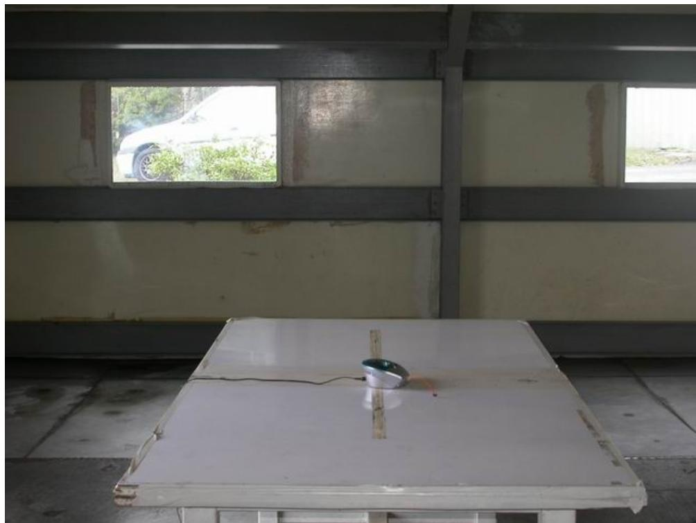
**POWERLINE CONDUCTED EMISSIONS MEASUREMENT SETUP**
