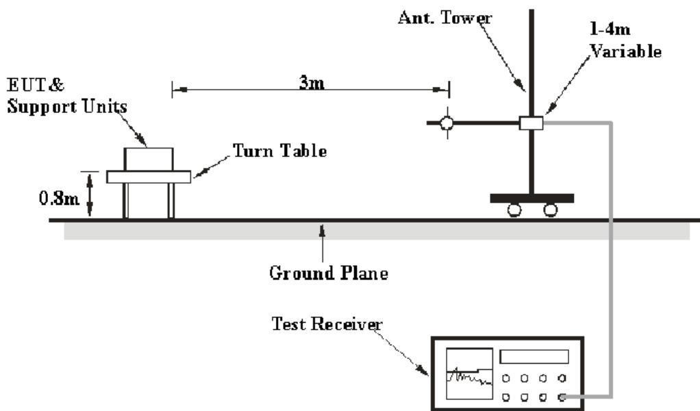
The radiated emission and out of band emission tests were performed in the 3 meters, using the setup accordance with the ANSI C63.4-2003. The specification used was the FCC 15.209 and FCC 15.249 limits.
