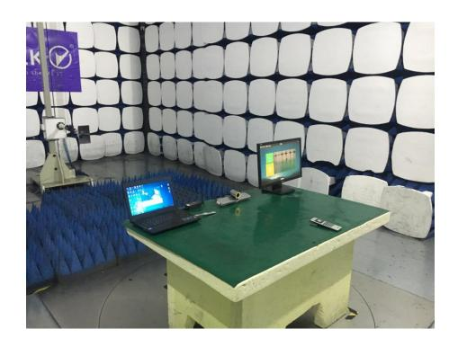
**Radiated Spurious Emissions Test**
