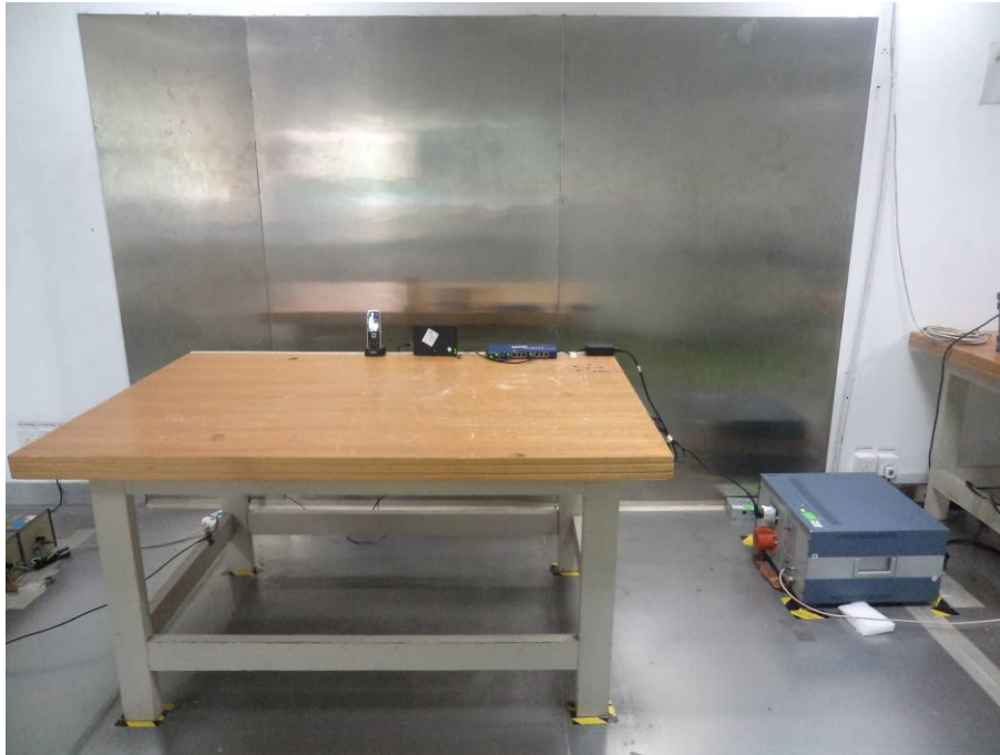
Conducted Emissions - Front View (PoE power)
