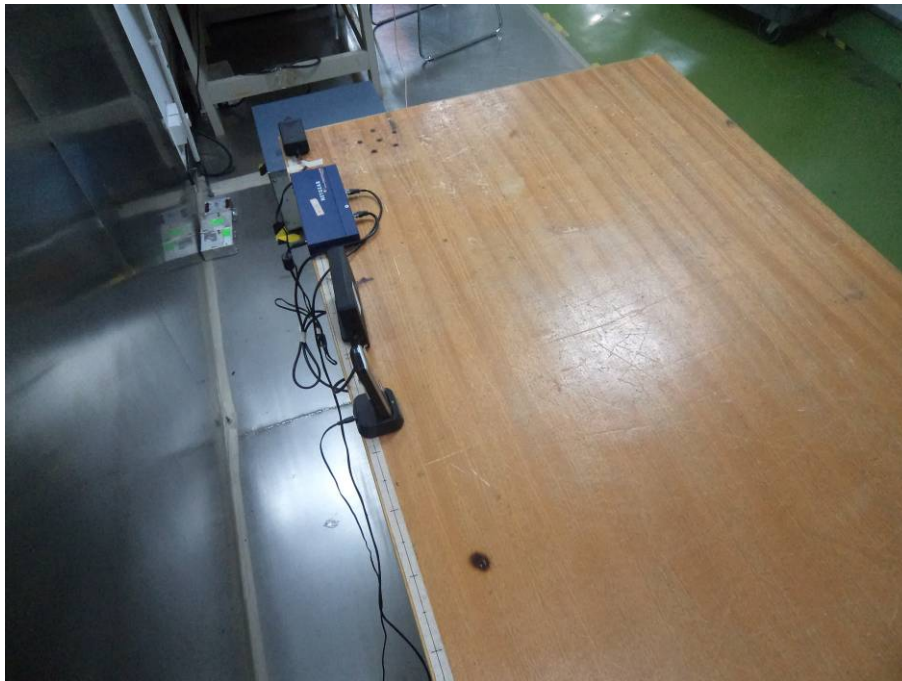
Conducted Emissions - Side View (PoE power)
