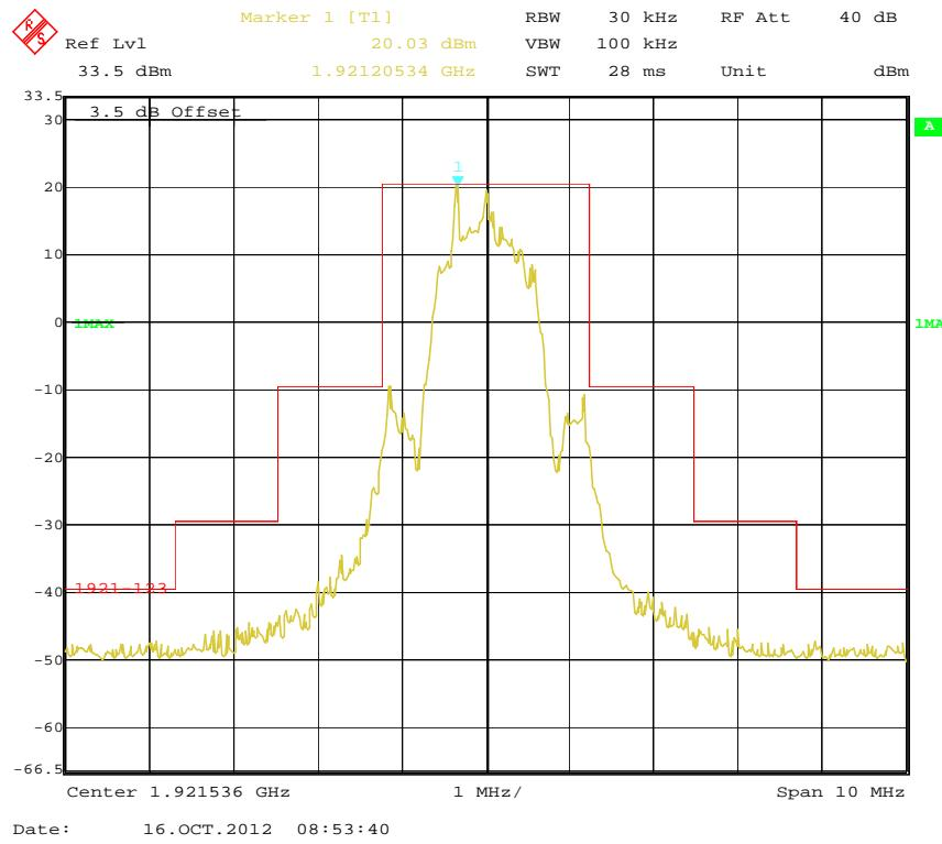
**Middle Channel (Unwanted Emission inside the Sub-band)**
