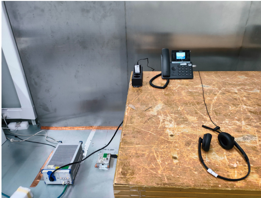
Conducted Emissions - Front View
