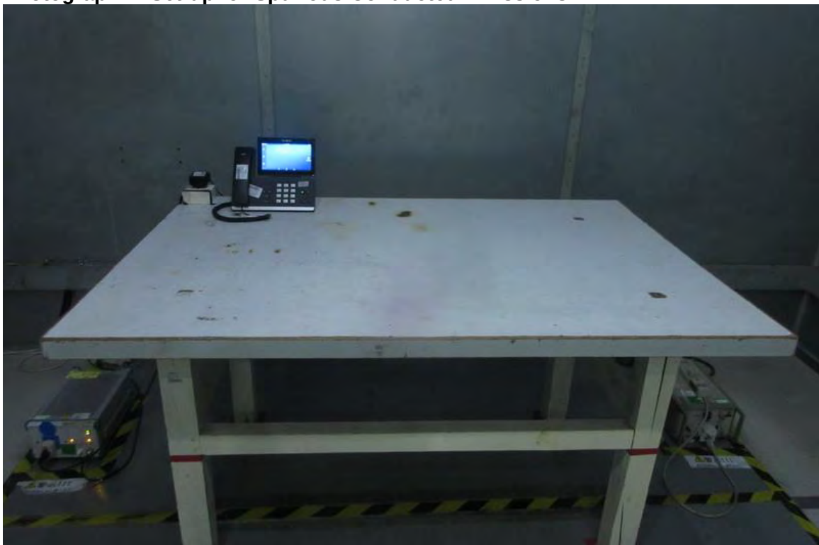
Photograph 4: Set-up for Spurious Conducted Emissions
