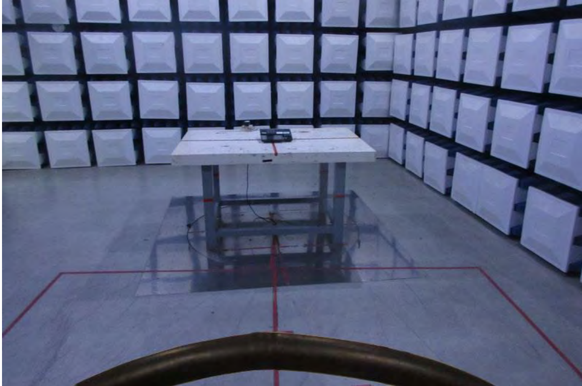
Photograph 2: Set-up for Spurious Emissions for 30 - 1000MHz
