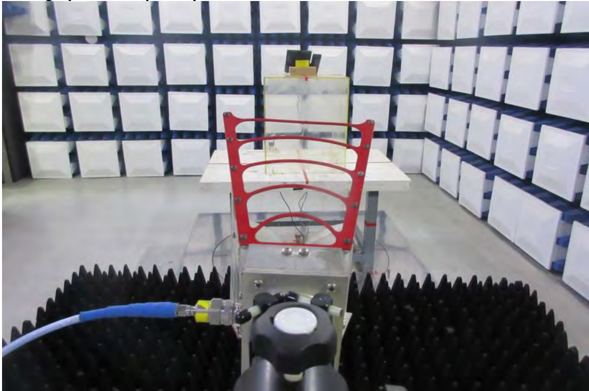
Photograph 4: Set-up for Spurious Conducted Emissions
