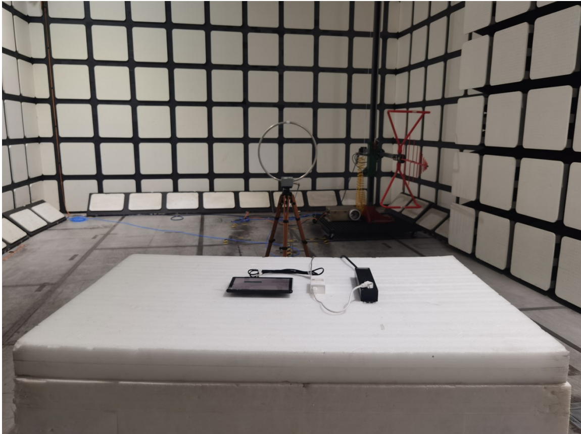
Radiated Emissions View (Below 1 GHz) POE
