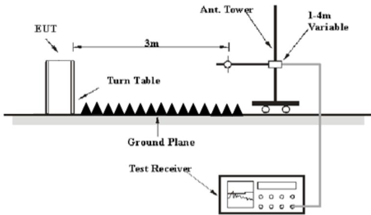
The radiated emissions were performed in the 3 meters distance, using the setup accordance with the ANSI C63.10-2013. The specification used was the FCC 15.209, and FCC 15.247,RSS-247,RSS-Gen limits.
