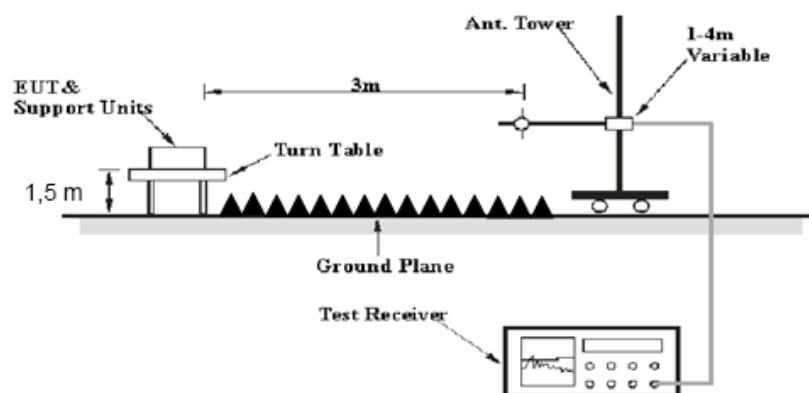
The radiated emission below 1GHz tests were performed in the 10 meters chamber test site, above 1GHz tests were performed in the 3 meters chamber test site B, using the setup accordance with the ANSI C63.10-2013. The specification used was the FCC 15.209, and FCC 15.247 limits.
