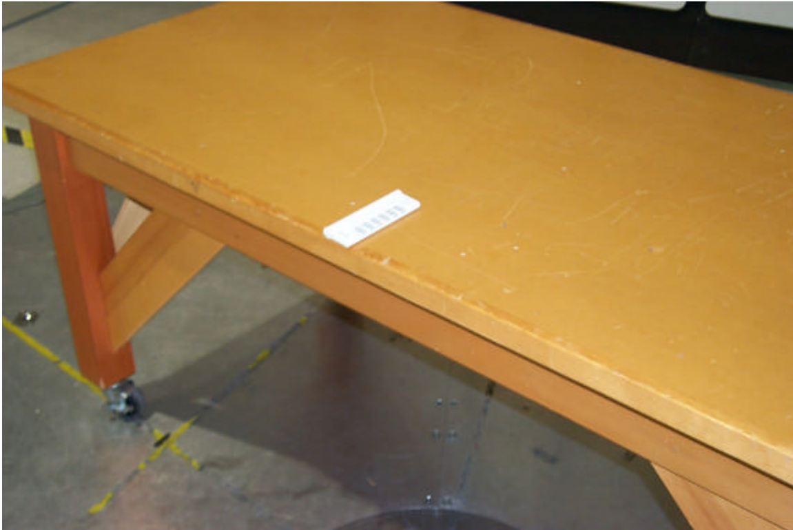
Figure 18 - Radiated Emissions Test Setup, EUT Horizontal (worst-case)
