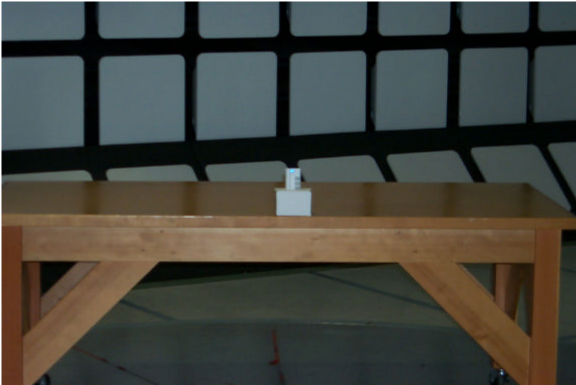
Figure 16 - Radiated Emissions Test Setup, EUT Vertical
