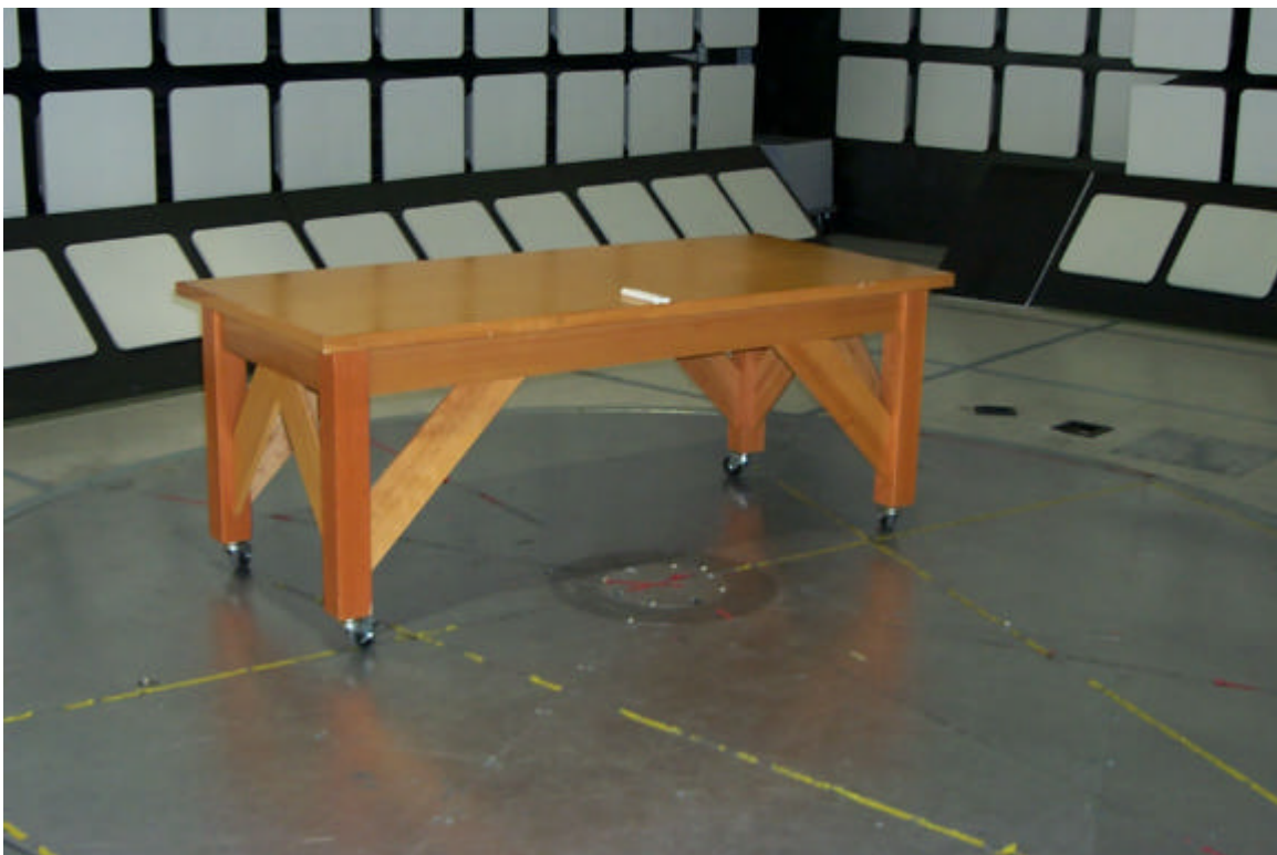
Figure 17 - Radiated Emissions Test Setup, EUT Horizontal (worst-case)
