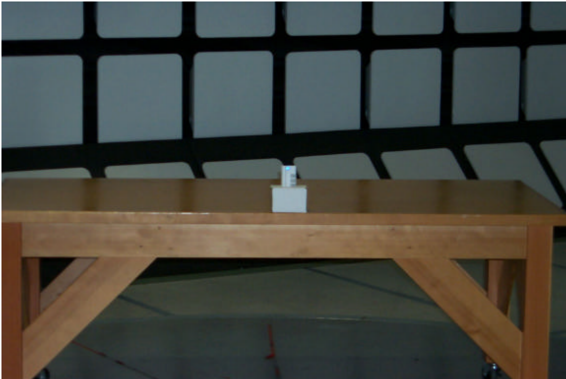
Figure 16 - Radiated Emissions Test Setup, EUT Vertical
