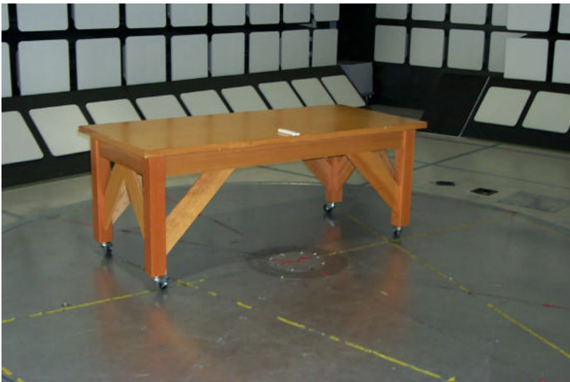
Figure 17 - Radiated Emissions Test Setup, EUT Horizontal (worst-case)
