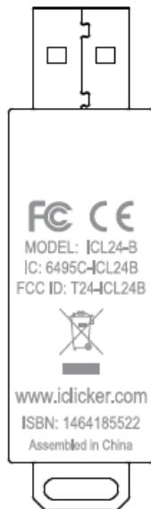
Label is pad-printed, or silk-screened, directly onto the base housing using acrylic ink. Scale 1:1
