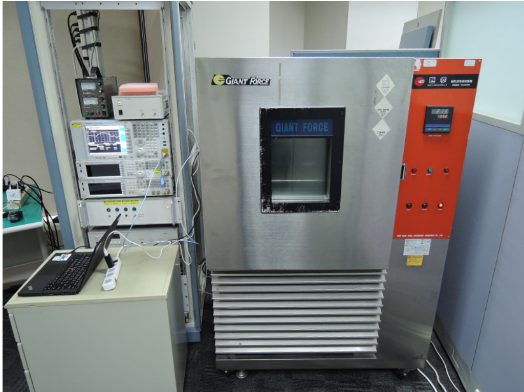
Photograph 6: Set-up for Mains Conducted testing (Back View)
