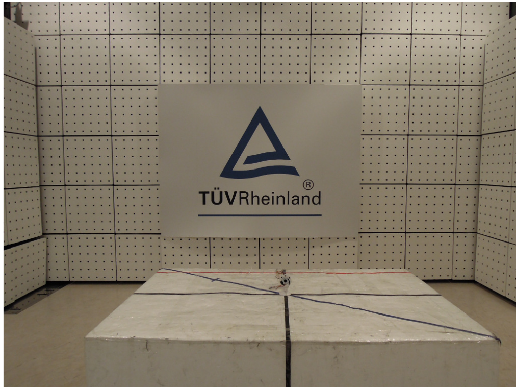
Photograph 1: Set-up for Spurious Emissions (Front View)
