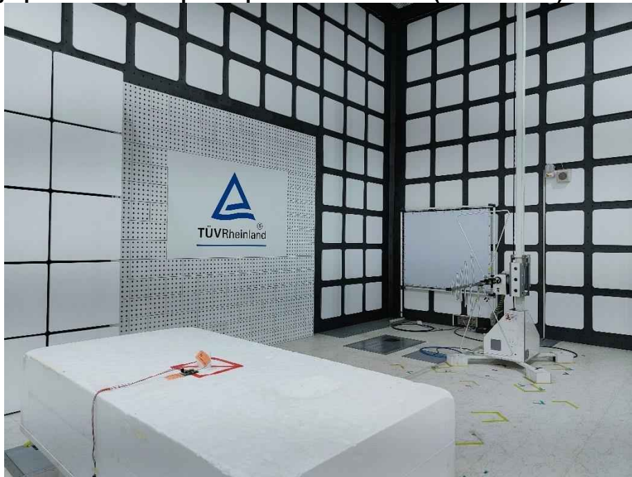
Photograph 12: Test Setup for Spurious Emissions (Back View 2)
