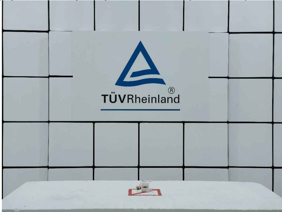
Photograph 9: Test Setup for Spurious Emissions (Front View 1)
