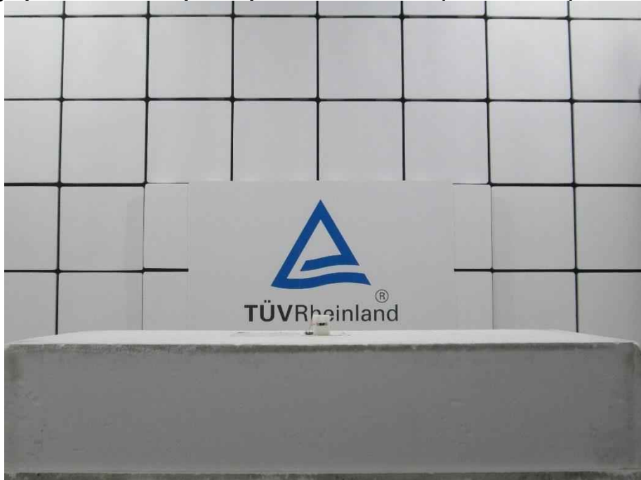
Photograph 10: Test Setup for Spurious Emissions (Front View 2)
