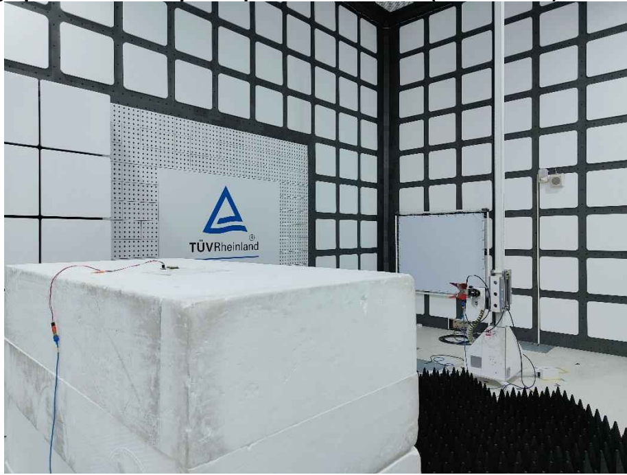
Photograph 30: Test Setup for Spurious Emissions (Back View 4)
