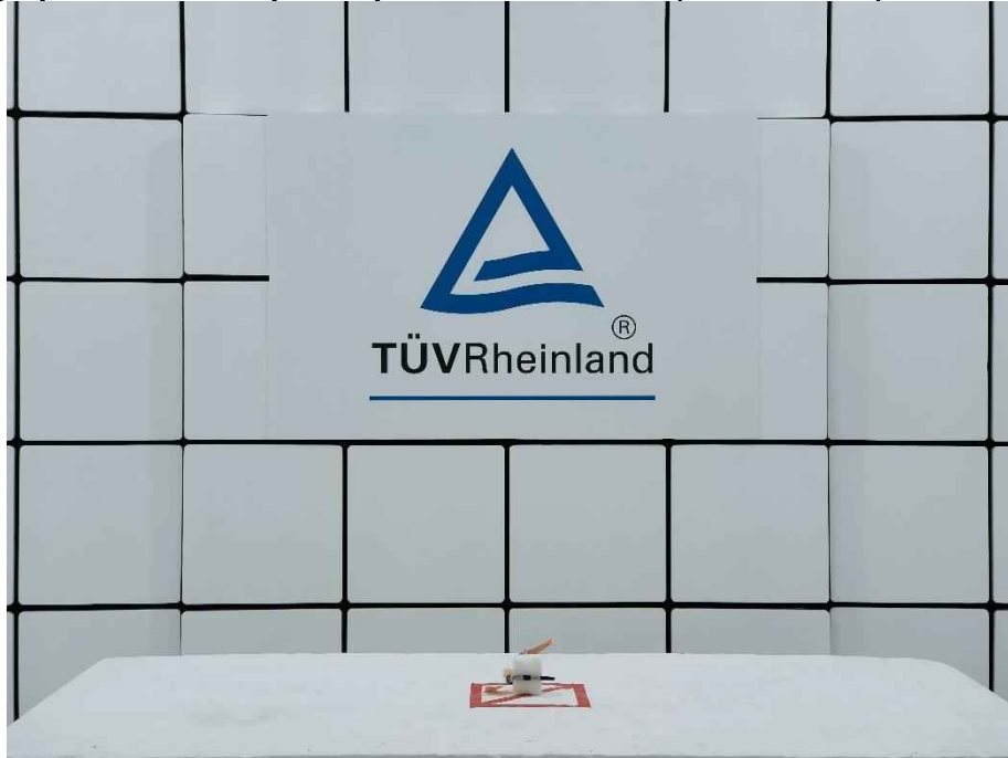
Photograph 1: Test Setup for Spurious Emissions (Front View 1)
