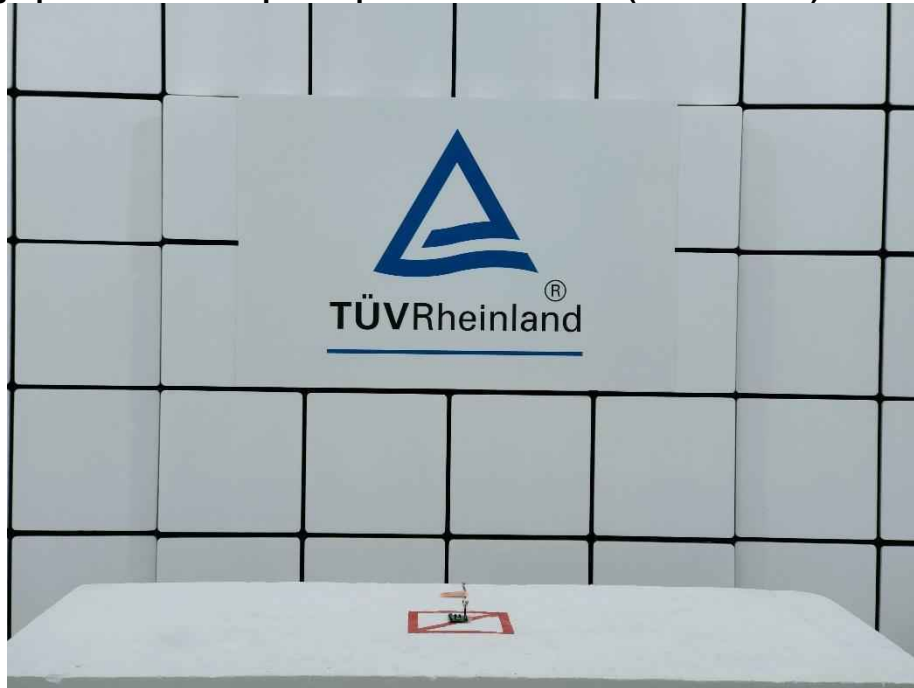
Photograph 25: Test Setup for Spurious Emissions (Front View 1)
