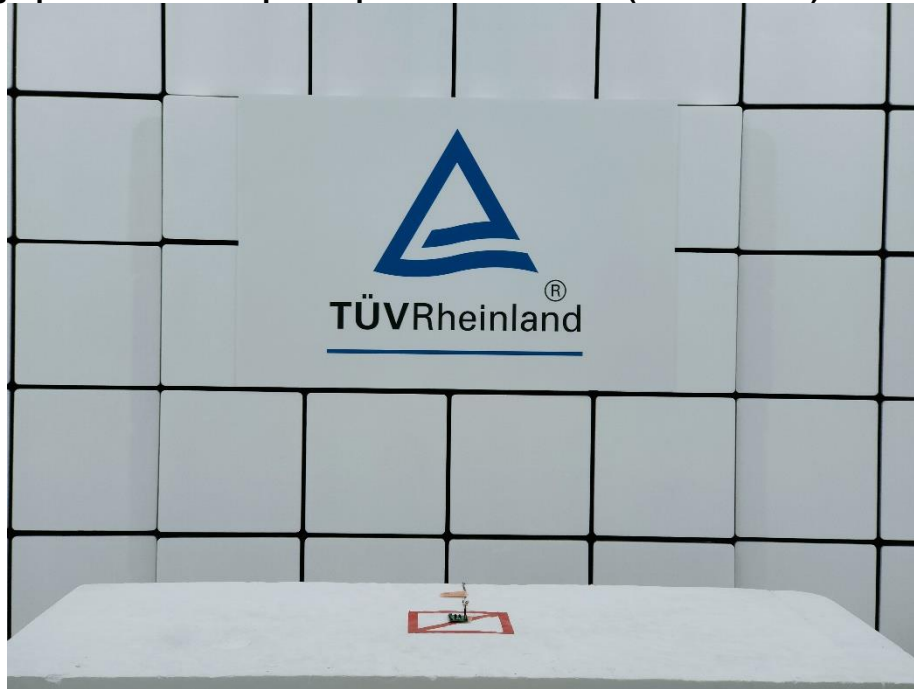
Photograph 26: Test Setup for Spurious Emissions (Front View 2)
