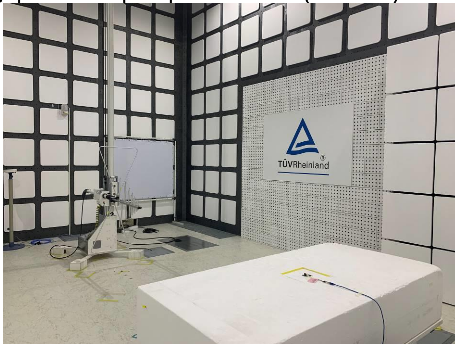
Photograph 4: Test Setup for Spurious Emissions (Back View 2)
