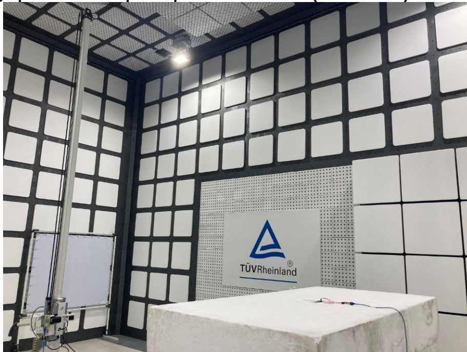
Photograph 6: Test Setup for Spurious Emissions (Back View 4)
