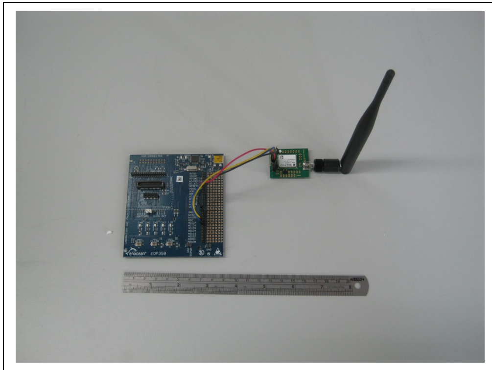
Photograph A3-1: Eval Board EOP 350, with EUT connected
