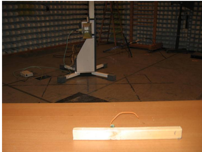
Figure 6-15: Test Configuration – Radiated Emissions (1GHz – 4GHz)
