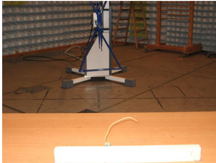
Figure 6-8: Test Configuration – Radiated Emissions (30MHz – 1GHz)
