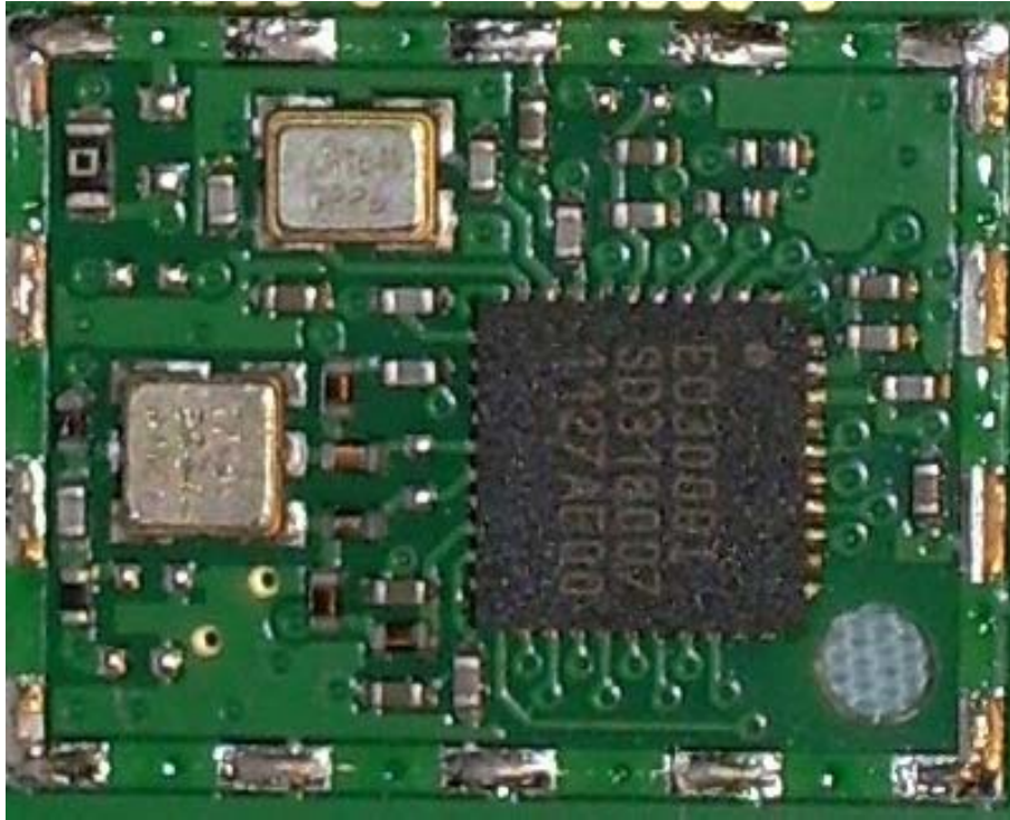
Photograph 6 – View of the Circuitry Under RF Shield
