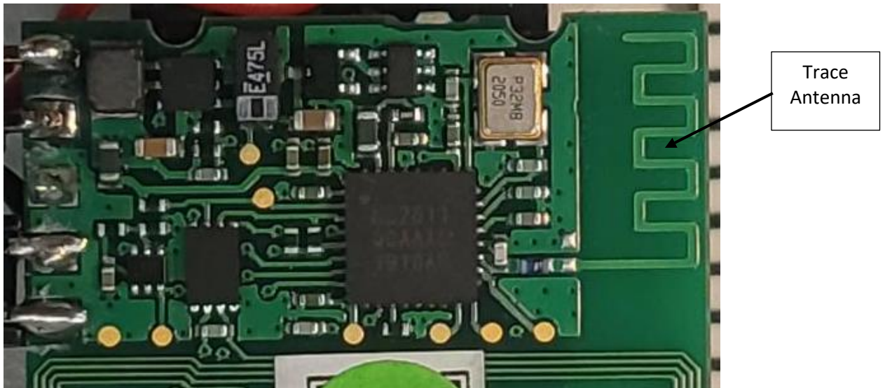
Photograph 1 – Close-up view of the RF Section
