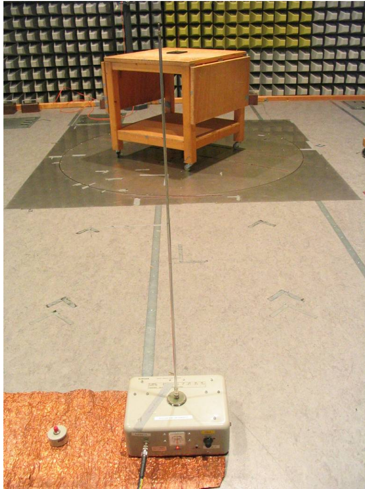
Figure 6-8: Test Configuration – Radiated Emissions (9kHz – 30MHz)
